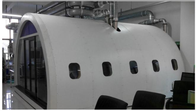
The laboratory mainly provides a platform for verifying the airworthiness of the cabin environment for civil aviation aircraft. Through the simulation and construction of the cabin air environment, it can simulate the actual aircraft cockpit air environment. The core parameters include temperature, pressure, humidity and pollution degree.
